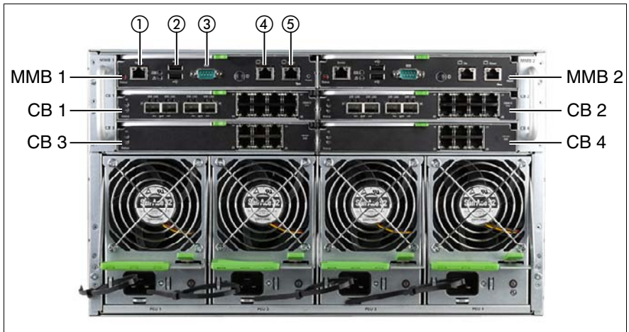
Figure 8: Ports for external devices (rack version)
